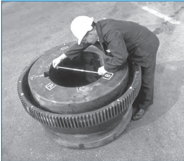
KOP-FLEX service technician inspecting gear coupling
