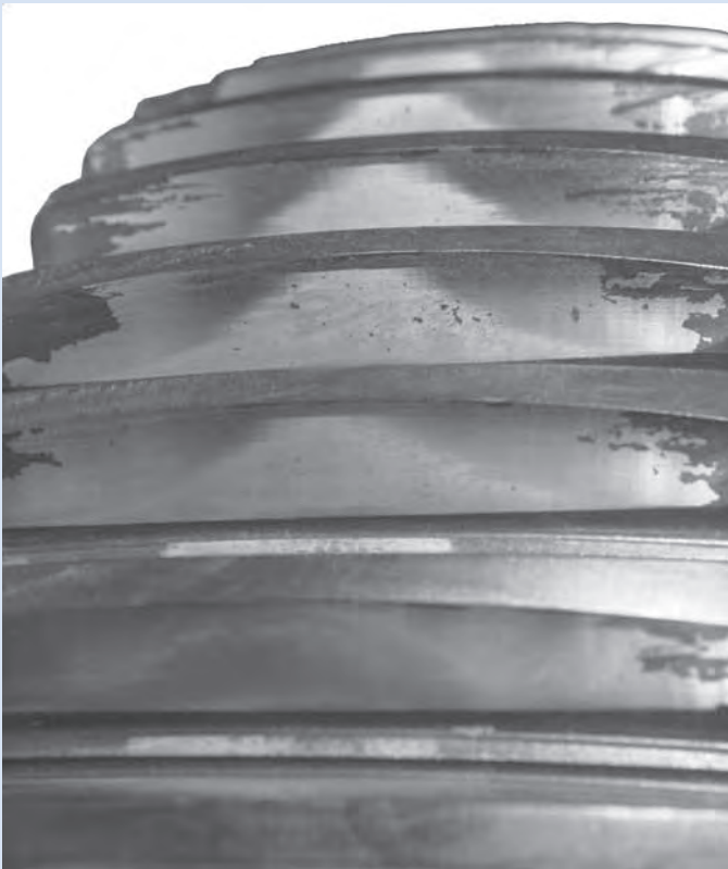
Contact Ground Gear (CGG) with contact check at 3° 90-100% Gear Tooth in Contact Excellent gear tooth flank finish
