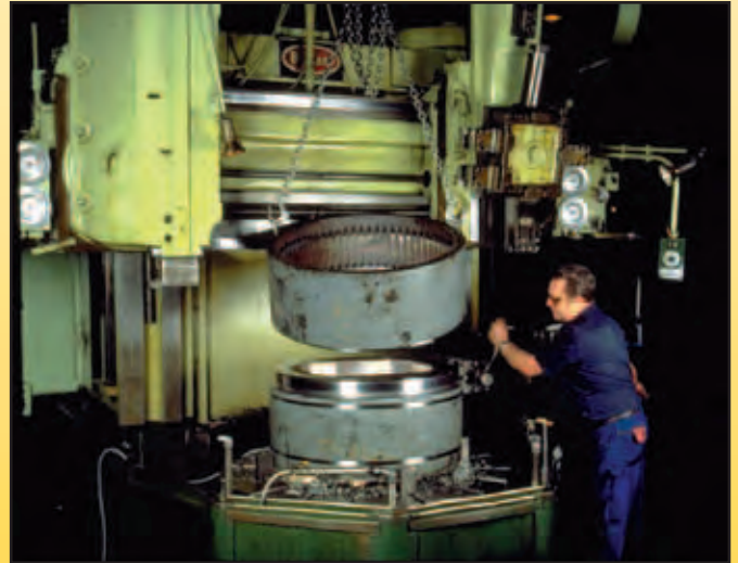
A damaged gear ring is machined off a spindle roll sleeve; The cost to repair is typically about half the cost of replacement
